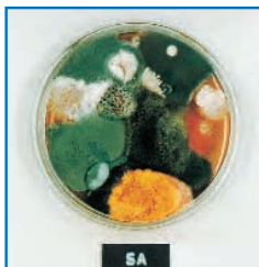
Microbiological swabs of insufficiently dewatered diesel samples
